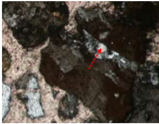
Figure (1) Photomicrograph showing silica cement (red arrow) in the sandstone of the Pondaung Formation.
