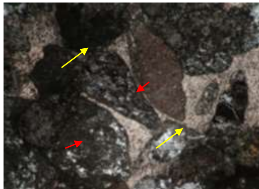
Figure (3) Thin section photomicrograph of sandstone from the Pondaung Formation showing calcite cement (red arrow). The calcite also replaced detrital framework grains (yellow arrow).
